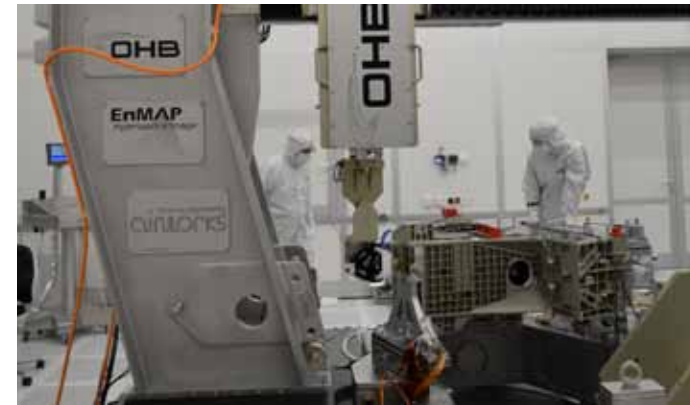
EnMAP IOU Flight Structure under dedicated Installation MGSE
