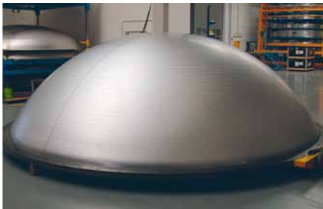
Partitions for tanks in the upper stage of next-generation launchers
