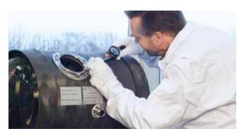
Water tank undergoing quality assurance at MT Aerospace
