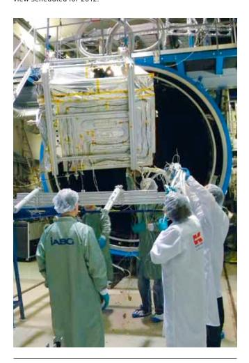
EnMAP before the thermal vacuum test at IABG mbH in Munich
